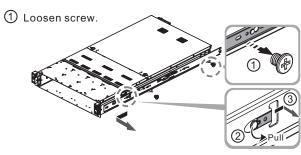
② Pull the latch upward and remove the keyhole from standoff and slide inner rail forward to remove inner rail.
